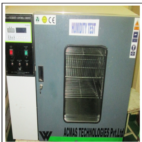
HUMIDITY CHAMBER (SPEC = 40C ± 5C AT 90-95% RH FOR 96 HRS)
