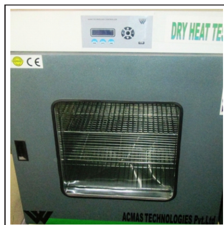
DRY HEAT CHAMBER (SPEC = 70C ± 5C FOR 96 HRS)
