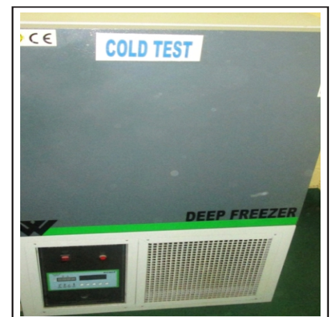
COLD CHAMBER (SPEC = - 20C ± 5C FOR 96 HRS)
